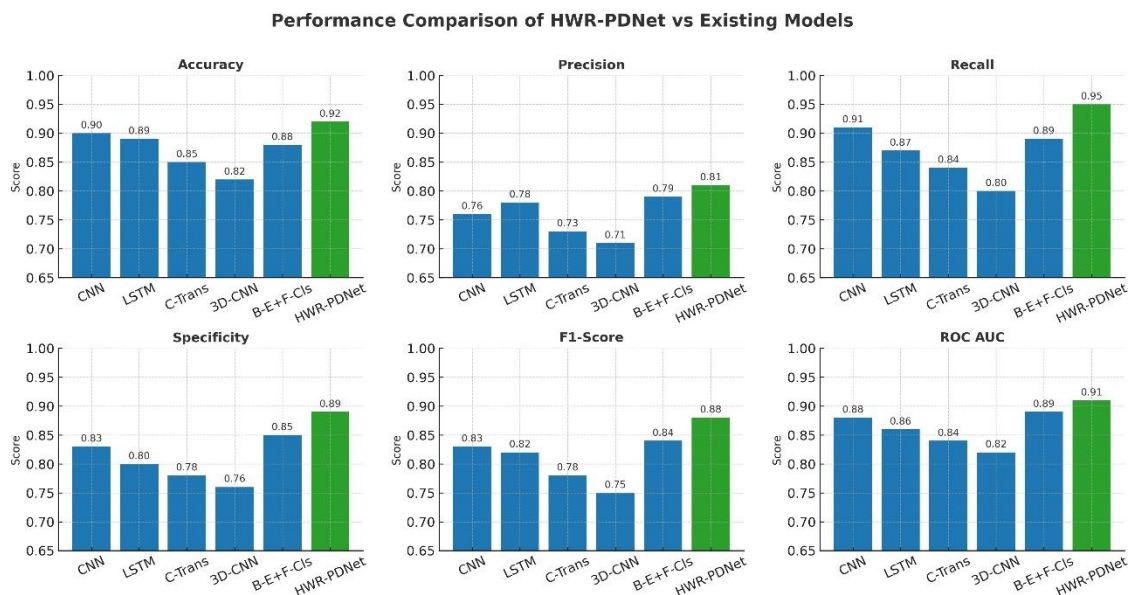
Figure 4. Performance comparison of HWR-PDNet vs. existing models' performance on the test dataset.
