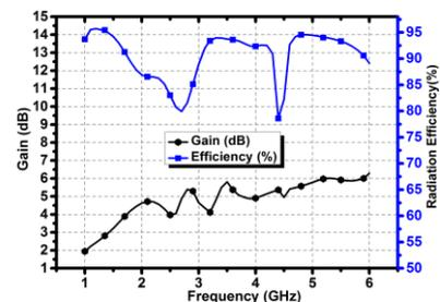
Figure 8. Gain and efficiency of the suggested antenna.
