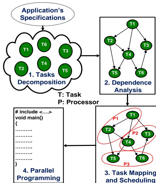
Figure 1. Task mapping and scheduling concept.
